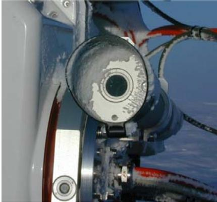
Cavity radiometer (direct solar radiation).
