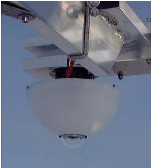
Precision Infrared Radiometer (PIR)
