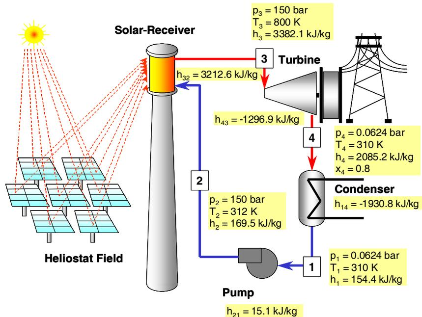
$$4) \quad \dot{W}_{el} = \dot{W}_{Turbine} - \dot{W}_{Pumpe} = (|h_{43}| - |h_{21}|) \dot{m} \rightarrow \dot{m} = \frac{\dot{W}_{el}}{|h_{43}| - |h_{21}|} = \frac{10 \text{ MW}}{(1296.9 - 15.1) \frac{\text{kJ}}{\text{kg}}} = 7.80 \frac{\text{kg}}{\text{s}} = 28.1 \frac{\text{t}}{\text{h}}$$
